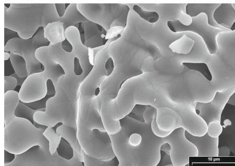
Figure 2: Microporosity in detail, pores up to approx. 5 µm; sinter necks are discernible.
