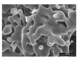
Figure 2: Micropores in detail, approx.  $5 \mu m$ , sinter necks are visible
