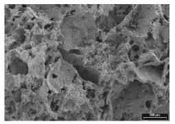
Figure 1: Macropores up to 500 µm are visible.
